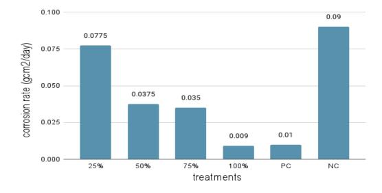
Mean corrosion rate of each treatment immersed in 1M NaOH
